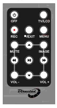
**NOTE:** This remote control does not function if the unit is docked in a overhead video unit. Use the overhead console's remote.
